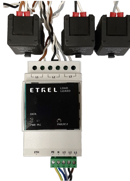
Figure 5: Load Guard with connected measuring current transformers
